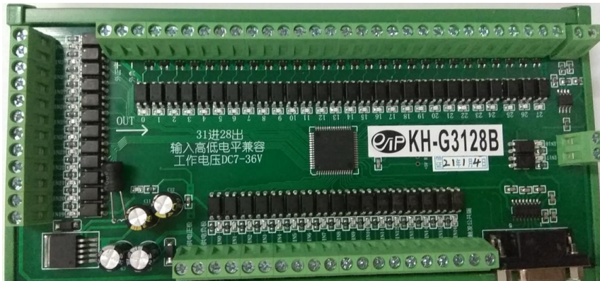
Figure 1.1.3a FAMIO Control Card KH-G3128B Upgrade Version: Compatible with both High and Low Level Inputs Appearance Diagram
